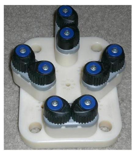
Fig. 10.2. Final Prototype of Knot-Tying Device.
