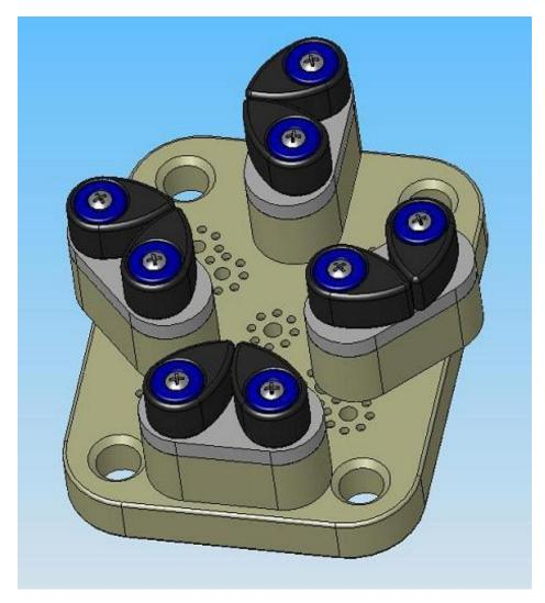
Fig. 10.1. CAD Model of Knot-Tying Device.
